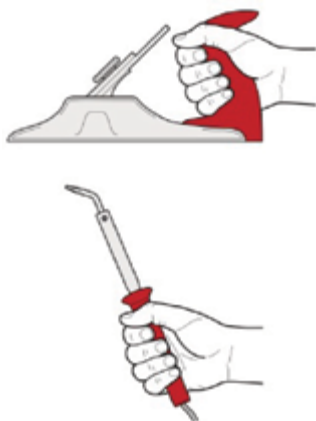
Figure 27 Select tools that can be held with a neutral wrist or in a handshake position with the hand adopting a comfortable, not too open or too closed, grip. Orient jigs and fixtures holding the work piece so the wrist does not have to bend.
