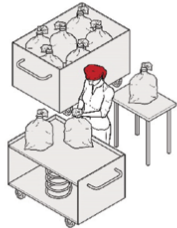
Figure 37 Self-adjusting base in laundry tubs reduces the need for bending, twisting and reaching during unloading.
