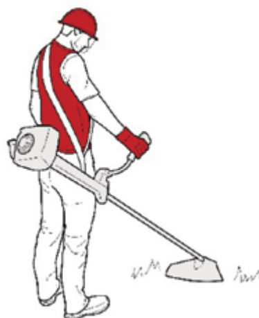
Figure 31 Weight supported by a harness; heaviest part of the brush cutter located behind the wrists
