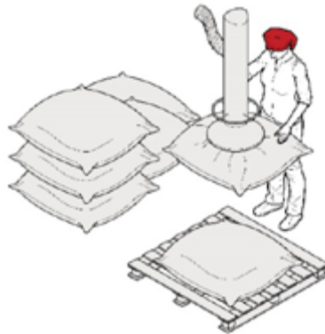
Figure 36 Vacuum operated lifting devices can reduce the forces, awkward postures, and movements required to manually load products onto pallets.
