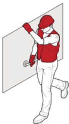
Figure 26 Use handling grip devices adapted to the particular object to be carried
