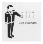
**Direct contact** refers to a person coming into contact with a conductor which is live in normal circumstances.
