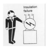
**Indirect contact** refers to a person coming into contact with a conductive part which is not normally live, but has become live accidentally due to insulation failure or some other cause.
