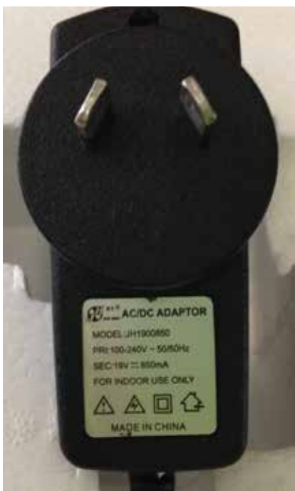
Power supply for mini laser stage lights
