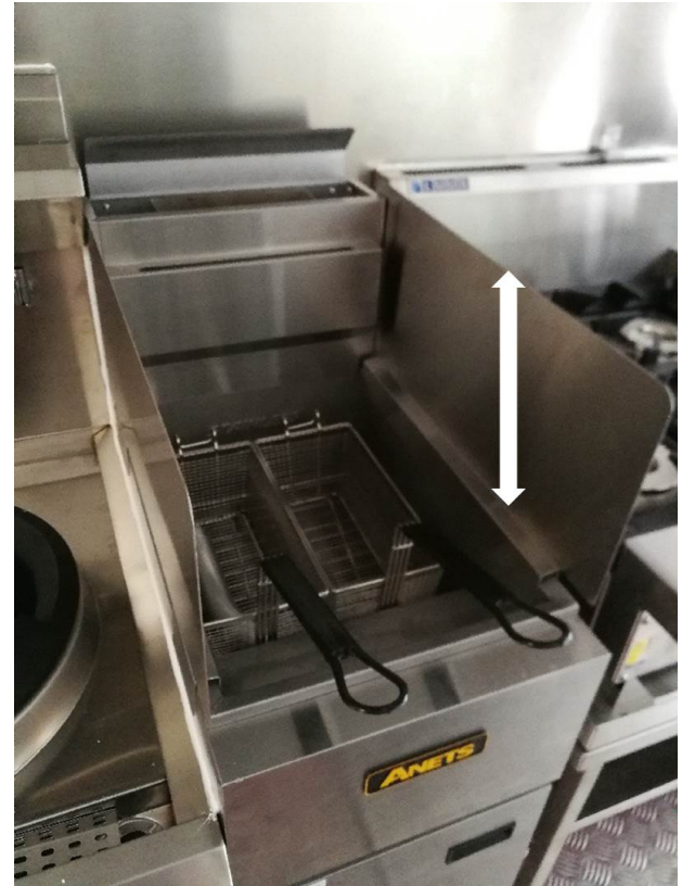
200mm minimum vertical baffle plate between fryer, wok burner to the left and boiling burners to the right
