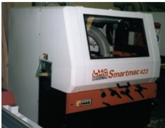
▲ Multi-surface moulder with cutters fully enclosed.
