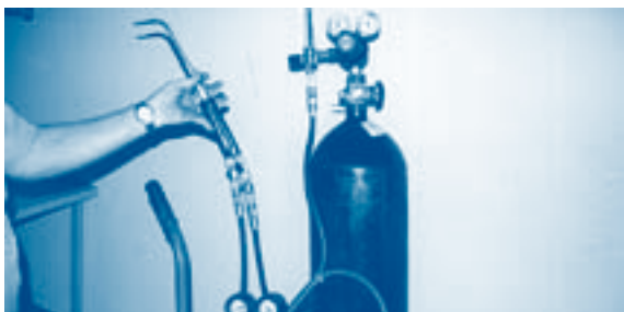
▲ Flashback arresters fitted to portable gas welding equipment.
