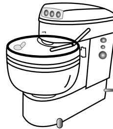
Examples of mixers with wire or solid guarding
