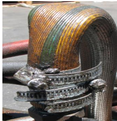
Secured Outlet Hose
