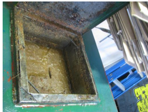
Figure 2: Example of clogged sieve in oil disposal machine (viewed from above)
