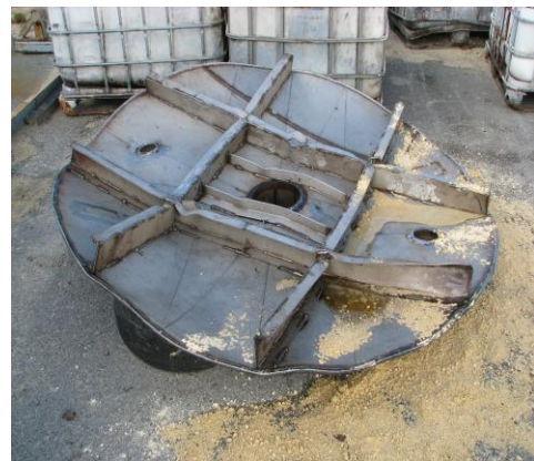
Photograph 1: This tank lid was blown off in the incident.
