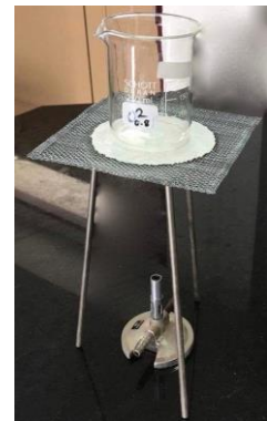
Figure 1: Bunsen burner mat sitting on tripod. The asbestos has been identified within the circular ceramic mat in centre of the mesh.
