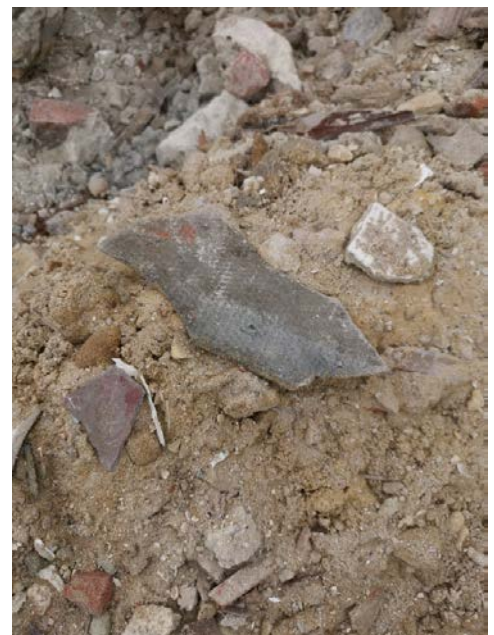
Figure 1: Asbestos-containing debris at a demolition site
