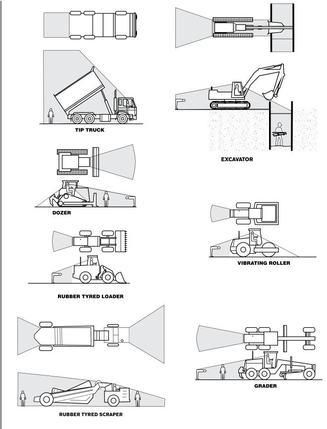
Figure 13: Dangerous shadows. Blind spots where operators may not see ground personnel
