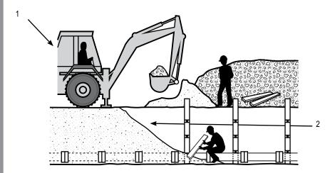
The trench should be backfilled to the level of the bottom tom before the tom is removed.
