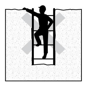
Figure 7: Worker climbing on trench supports.
