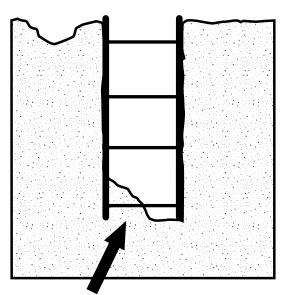
Figure 5: Waterswelling or uplift of the trench bottom.
