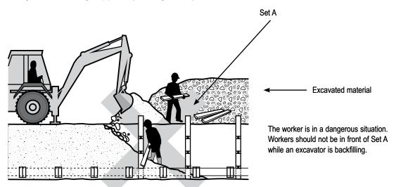
Figure 11: Worker in trench outside the support system.
