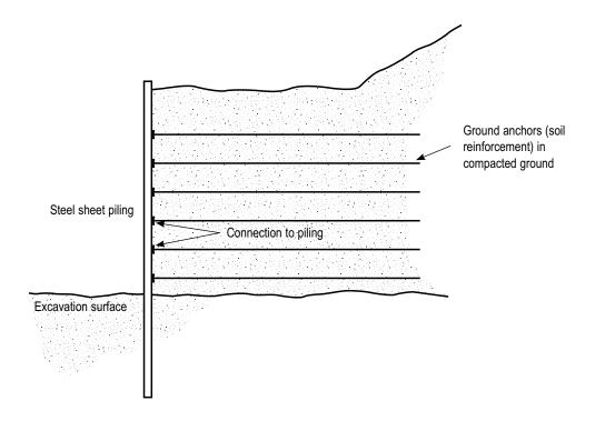
Figure 27: Ground anchors – for supporting steel sheet piling.
