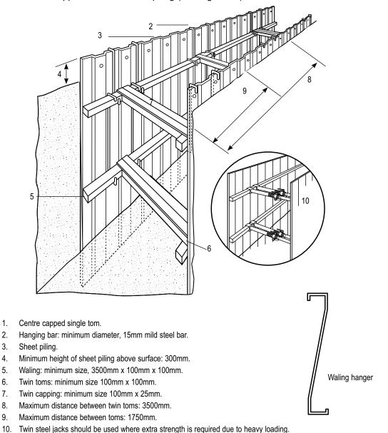
Figure 26: Sheet piling in unstable ground. Sheet piling may be used when ground is so unstable that side wall collapse would be likely immediately after excavation, for example, in loose and running sand. In such cases, sheet piling needs to be carried out before excavating.
