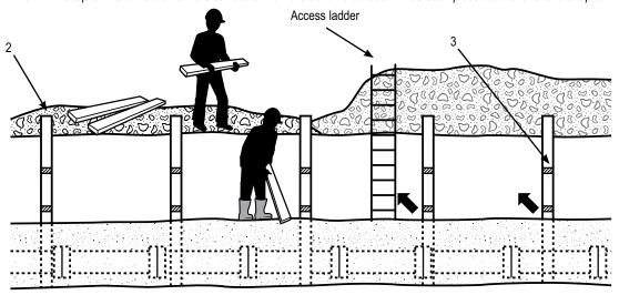
For added side support during the removal process, while workers are still in the trench, the soldiers should be left in place until all the toms have been removed, and then extracted with a backhoe.
