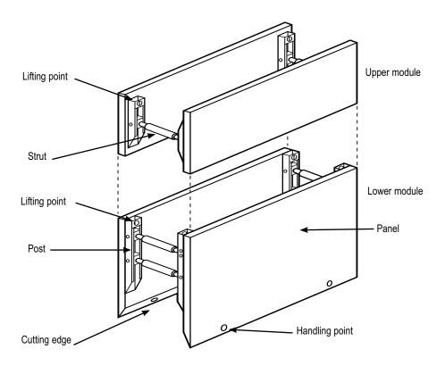
Figure 23: Typical trench shield.
