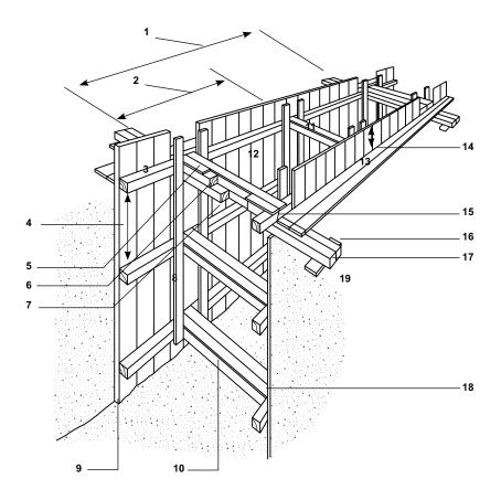
Figure 18: Closed sheeting; vertical timber trench support in loose or running ground, for trenches with a maximum depth of 5.0 metres.
