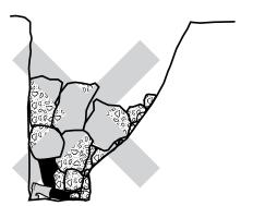
(d) Worker badly injured and probably smothered after being crushed against the opposite wall by the collapsing ground. The weight of a wedge of sand over a one metre length of trench two metres deep is about three tonnes; more than enough to crush a worker's chest.
