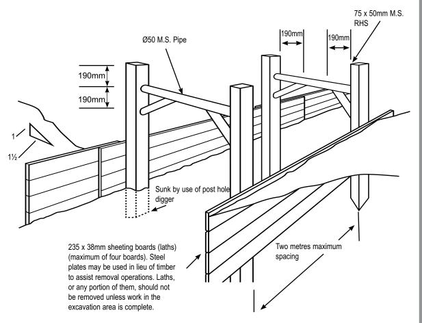
Figure 22: Trench support in sand. Steel soldier sets. Horizontal timber sheeting boards (side lacing). Maximum trench depth two metres.
