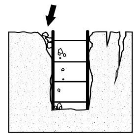
Figure 6: Surface soil falling into the trench.
