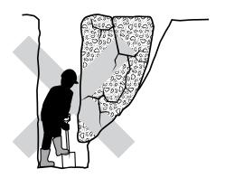
(b) Shear plane failure along the seepage (slippage) plane.
