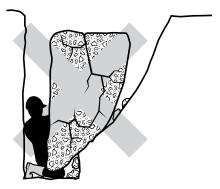
(c) Worker trapped and crushed against the trench wall by the quick collapse.
