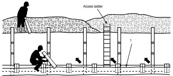
Trench should be filled to the level of the bottom toms before workers can be allowed into excavation to remove the bottom row of toms.
