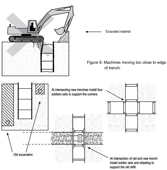
Figure 9: Trench in or near previously dug ground.
