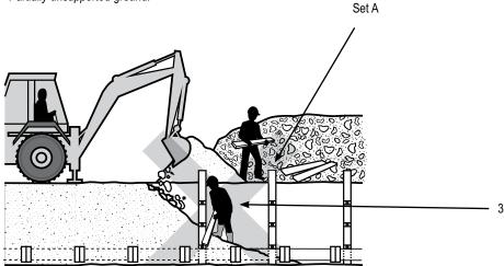
Since the soldier provides side-support near the set being dismantled, the set should be removed by the backhoe only after the trench has been completely backfilled.
