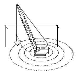
High voltage contact will result in electrical current flowing down the boom and through the machine to the ground. The ground will then be energised with a high voltage near the machine and lower voltage further away.
