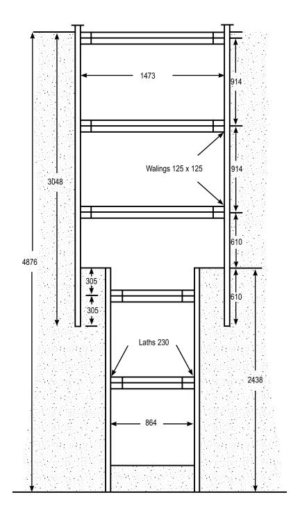
Figure 19: Sketch of telescopic set. All measurements are in millimetres (not to scale).
