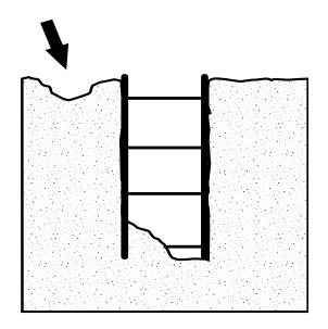
Figure 4: Subsidence alongside the trench.
