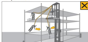
Figure 4 A lanyard or inertia reel that is too long can result in the 'pendulum effect'
