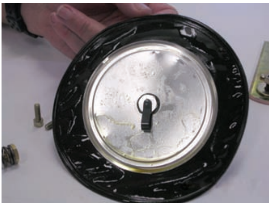
After running only 1661 km on LPGas this vehicle could no longer run on LPGas. This wetted and jellified diaphragm covered in plasticiser residue was obtained from this vehicle.
