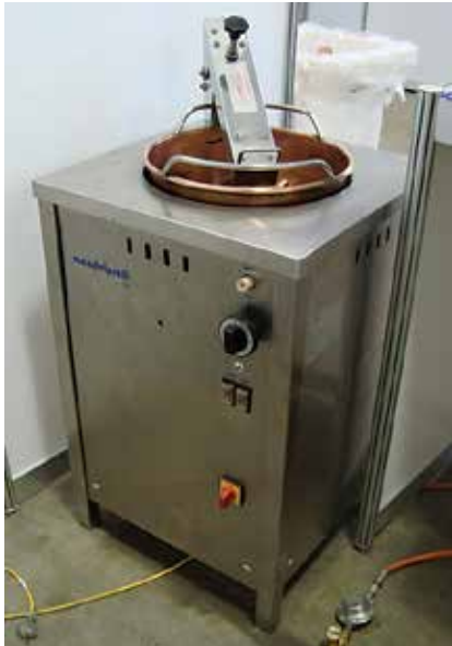
Unapproved high pressure propane appliance.
