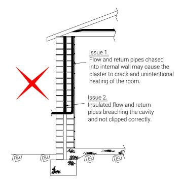
Diagram 2: Issues with flow and return lines serving solar panels
