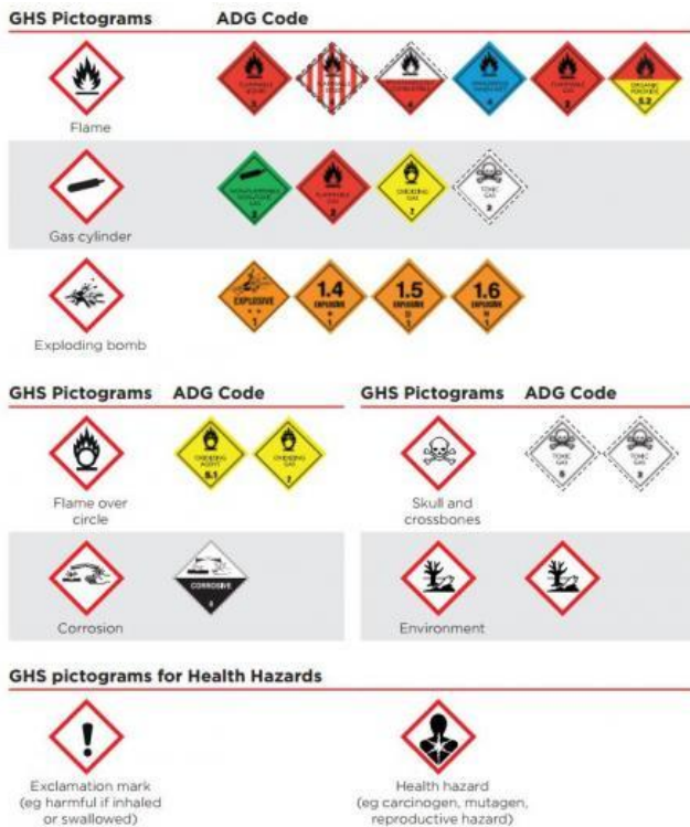
Comparison between GHS hazard pictograms with the corresponding ADG Code labels, by Safe Work NSW.
