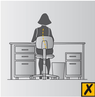
A8 – Inadequate leg clearance
