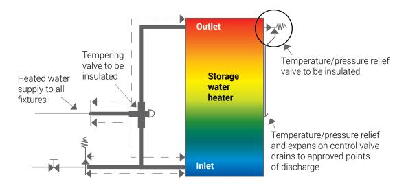
NOTE: Insulation for a minimum of 500 mm measured along the pipe as indicated by dashed lines
