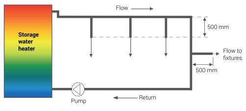
**NOTE:** All flow and return pipes fully insulated
