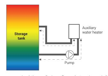
NOTE: Insulation on all primary flow and return pipes as indicated by dashed lines
