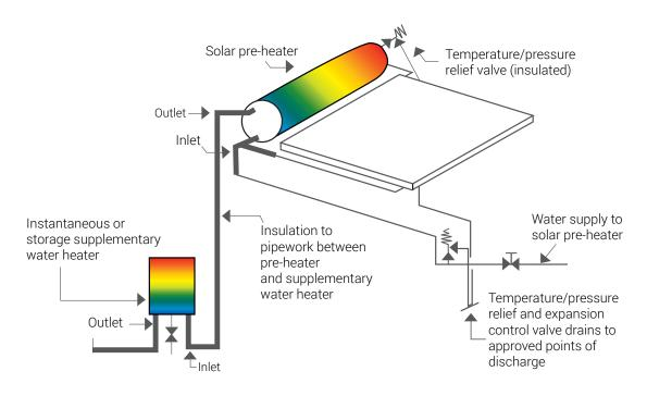
**NOTE:** Insulation required on cold water inlet piping for storage water heater
