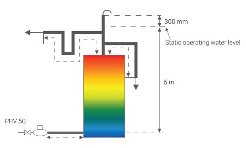
**NOTE:** Insulation for a minimum of 500 mm measured along the pipe as indicated by dashed lines
