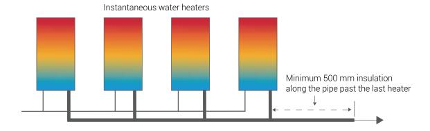
**NOTE:** Insulation for a minimum of 500 mm measured along the pipe as indicated by dashed line Insulation required on cold water inlet piping for storage water heaters
