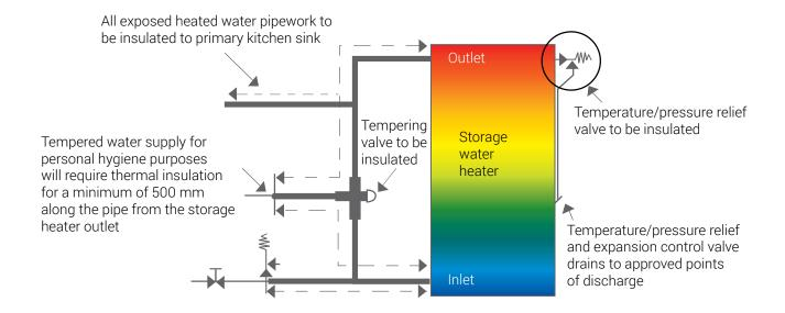
**NOTE:** Insulation for a minimum of 500 mm measured along the pipe as indicated by dashed lines All valves to be insulated if within 500 mm from the storage water heater
