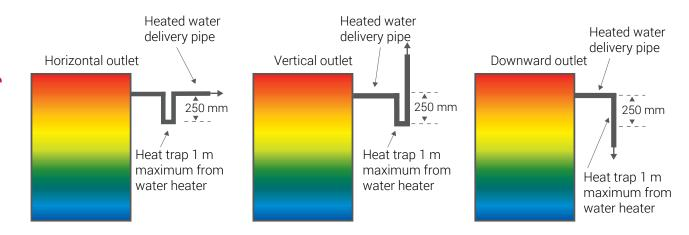
Diagram 11: Heat traps on storage water heaters
