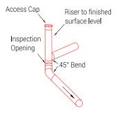
**Diagram 6:** Preferred method of providing raised access into drain
