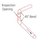
**Diagram 5:** Preferred method of providing access into drain
