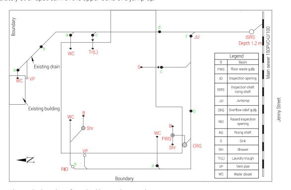
**Diagram 1:** Shows the location of required inspection openings
