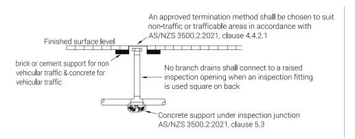
Diagram 2: Typical raised inspection opening
