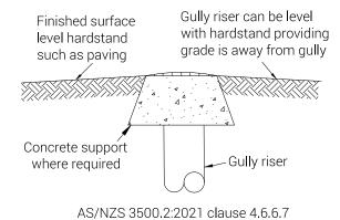
**Diagram 15:** Typical gully riser termination in paved non-traffic areas
