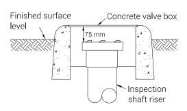
**Diagram 13:** Typical inspection shaft riser termination with valve box in non-traffic areas
