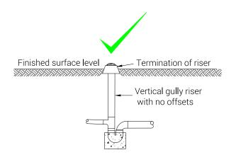
Diagram 7: Compliant disconnector gully
