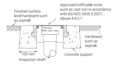
**Diagram 16:** Typical inspection shaft riser termination in areas subject to vehicular traffic
