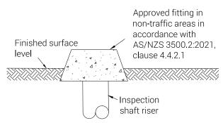
**Diagram 14:** Typical inspection shaft riser termination using an approved fitting in non-traffic areas
