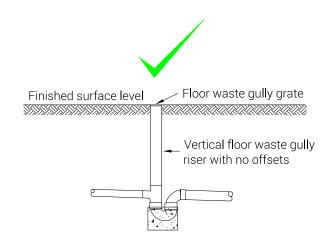
Diagram 8: Compliant floor waste gully
