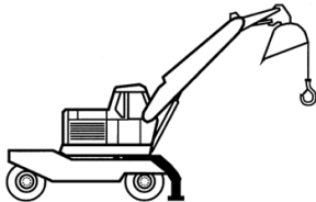
Figure 1 - Earthmoving machine with lifting device
