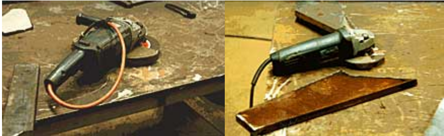
Photo 1. nine inch grinder (left) is noisier than four inch one ( right)
