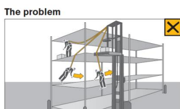
Figure 4 A lanyard or inertia reel that is too long can result in the 'pendulum effect'
