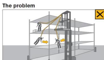
Figure 4 A lanyard or inertia reel that is too long can result in the 'pendulum effect'
