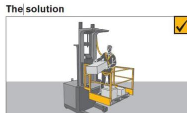
Figure 5 A fully enclosed platforms can prevent falls from an order picker.
