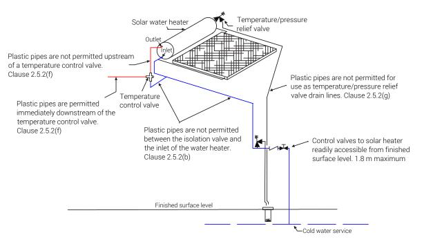
Diagram 1: Solar water heater cold water inlets and heated water outlets
