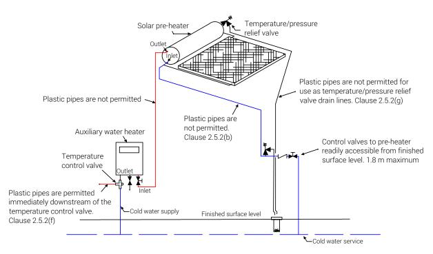
Diagram 3: Solar pre-heaters and auxiliary water heaters
