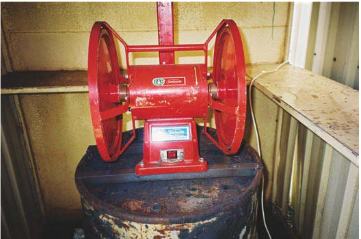
Grinders should be in a secure, properly lit enclosed space.
