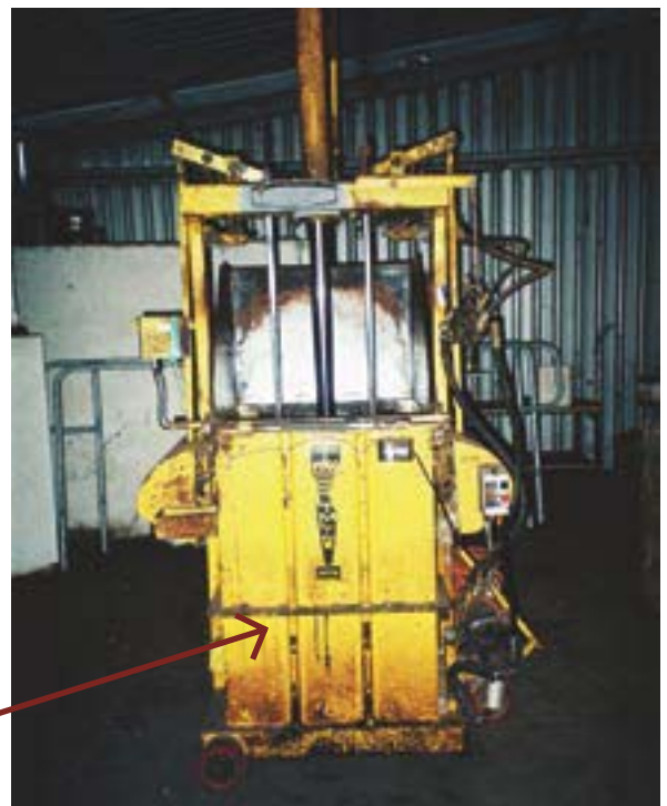
This well maintained wool press has a trip bar fitted.
