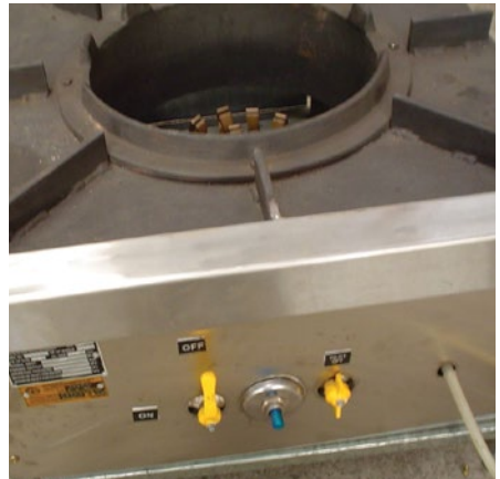
Individual and custom-built industrial gas appliance – pot cooker
